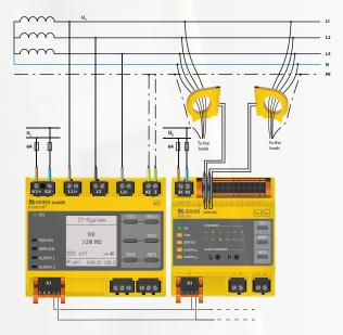
Insulation fault location systems (EDS) quickly identify the faulty part of the installation. Insulation fault location takes place during operation, shutting down the installation is not necessary. The information regarding the fault location is indicated at a central point.
