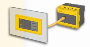
The display unit FP200 is mounted in the front using retaining clips and connected via a provided RJ45 connection cable to the basic devices without display. This installation variant makes it possible to install the display of the device in the control cabinet front without having to route the system connection with up to 1,000 V.
